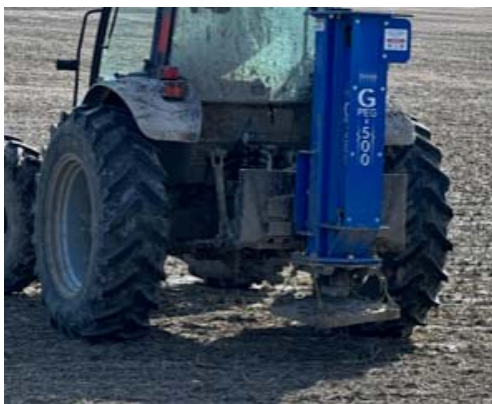
Please note the small plate at the bottom of the weight drop.
