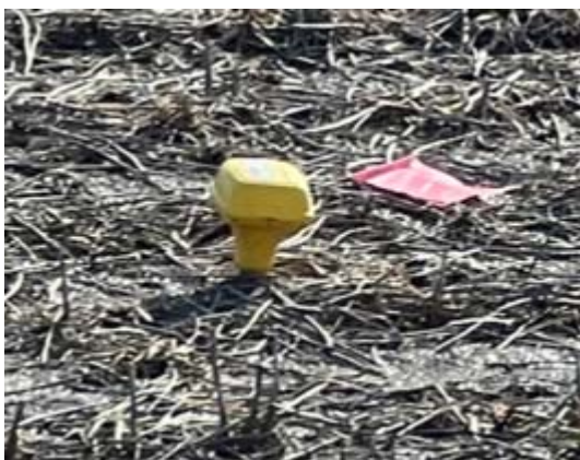
The wireless geophone is slightly bigger than a bar of soap.
