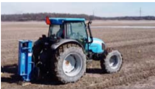
This is the testing vehicle with the weight drop behind.
