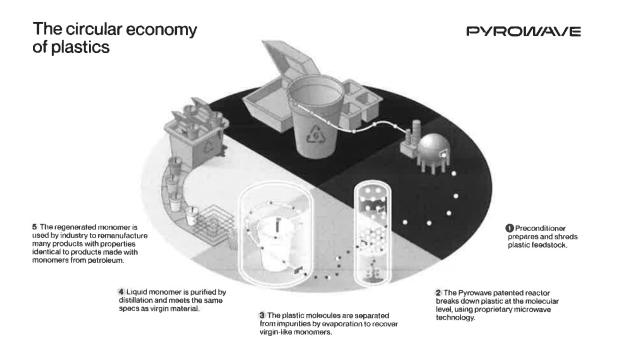
The Pyrowave technology platform uses microwaves to manufacture chemicals more efficiently and with a lower carbon release than traditional processes.
